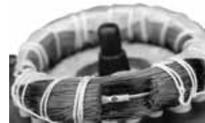
Fig. 21 PTC sensor incorporated in winding
