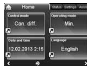
Fig. 106 Example of the main display on an NBE, NKE Series 2000 with an advanced operating panel
