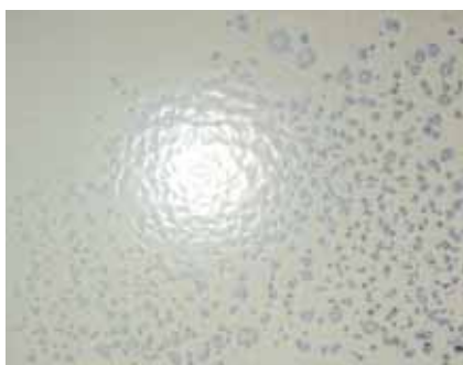
Fig. 94 Example of coated surface contaminated with PWIS
