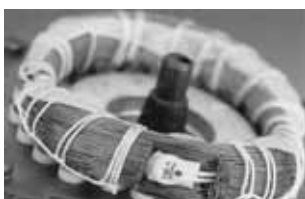
Fig. 23 Thermal switch incorporated in winding
